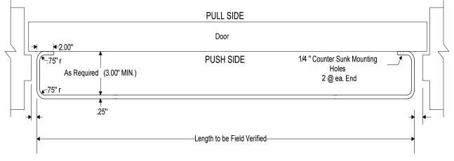
Specify: <sup>1</sup>/<sub>4</sub>" x 4" or <sup>1</sup>/<sub>4</sub>" x 6" 6061 T6 Aluminum Alloy (Anodized)
